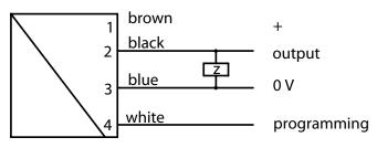
The correct supply voltage value acc. to datasheet values has to be obeyed prior to installation! The use of shielded cable is highly recommended, cable length < 30 m, supply lines < 10 m.
