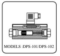
FILTER CLOG/D.P SWITCHES MODELS: DPS- 101/ DPS 102.
