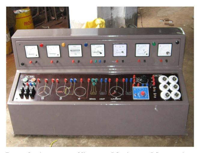
Features :Speed torque curves of Shunt motor, DC series motor, DC compound motor & Separately excited DC motor. -DC separately excited generator.
