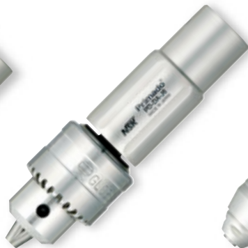
order code PD-DA-J6 Jacobs Keyed Drill Chuck • ø0.5~ø6.5 mm
