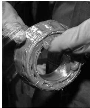
Fig. 23. Grease can easily be packed by hand.
