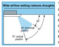
The wide vanes and the smudge-free airflow control mechanism work together to reduce smudging that normally appears on the ceiling and enable draughtfree cooling, enhancing comfort levels significantly.
