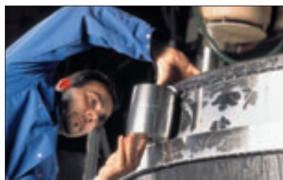
Checking of roller seats
