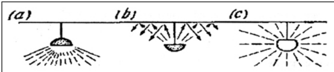
Light from luminaries can be (a) direct; (b) reflected; and (c) diffuse
